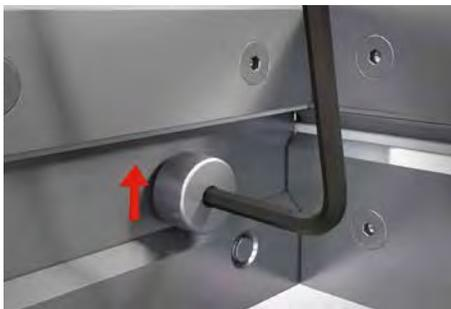
Externally-greased cam adjustable rollers allow for easy blade adjustments
