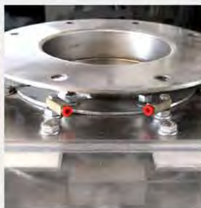
Air purge ports are used to reduce material migration between replaceable seals
