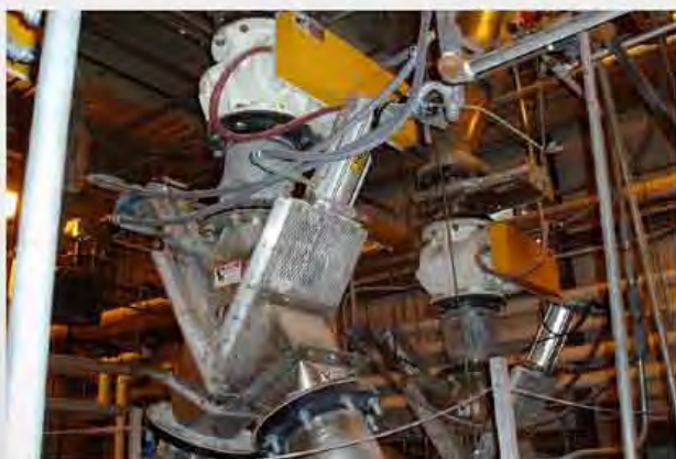
8" (203mm) Gravity Vee Diverter below a rotary valve handling zinc oxide
