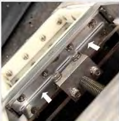
Braided Teflon packing seal gives positive material & air seal up to 15 PSIG to atmosphere in the open position
