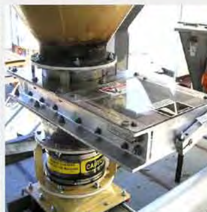
10" (254mm) Maintenance Gate handling PVC resin
