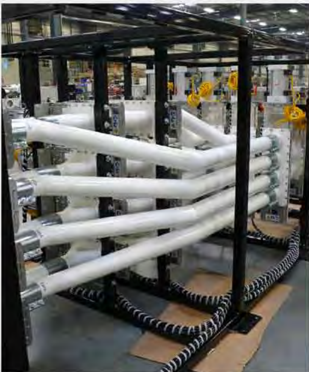
2 x 8 Multi-Port Diverter handling plastic pellets
