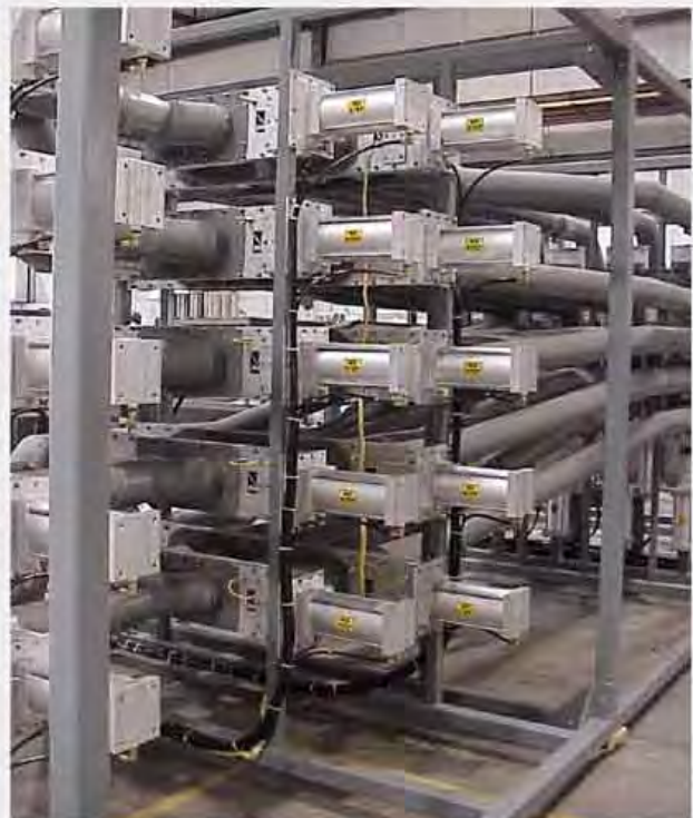
5 x 5 Multi-Port Diverter with all lines running simultaneously handling plastic resin
