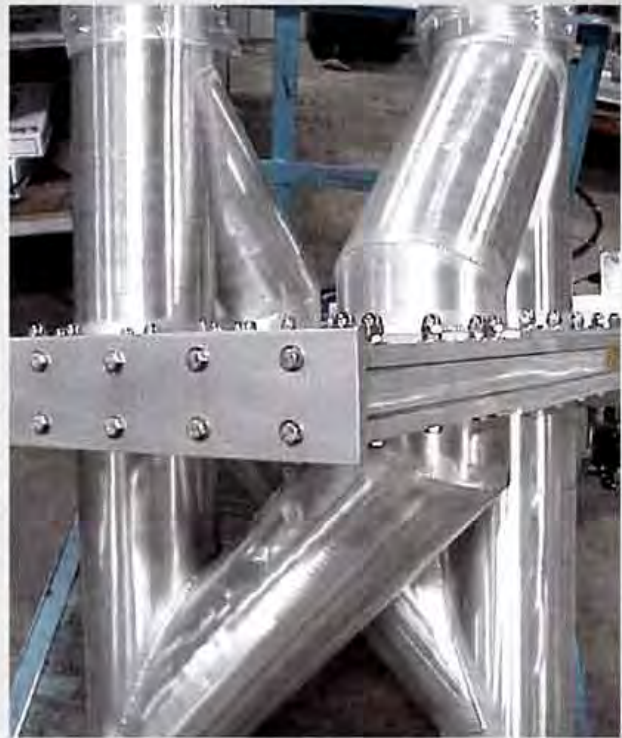
4" (102mm) Cross-Over Diverter handling titanium dioxide
