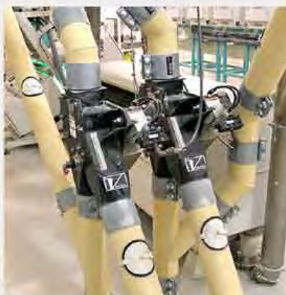
6" (152mm) Seal Tite Diverter handling flour
