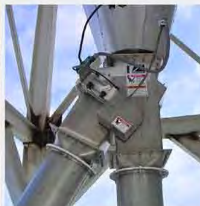
10" (254mm) straight line Seal Tite Diverter handling kaolin clay
