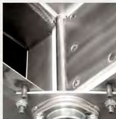
The shaft seal replaces the open area where migration of material to the off leg normally occurs
