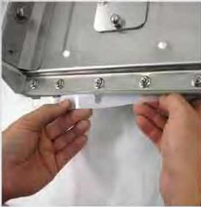
Shim removal for seal adjustment while valve is in-line
